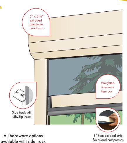
Hem bar hangs into side tracks 3¾" when retracted Pile top seal Hem bar behind screen 1" hem bar seal strip Side track with ShyZip zipper insert Oasis 2900 White **Bronze** Tan Black
