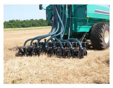
Figure A-17-2. Manure injection mechanically applies the organic nutrients – manure, bio-solids, or compost – into the root zone with surface soil closure at the time of application. This offers the greatest nutrient reduction and odor reduction due to limited soil disruption, amount of material left on the soil and immediate soil closure. Photo: Livestock and Poultry Environmental Learning
