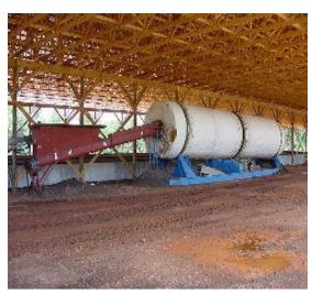
Figure A-14-3. In-Vessel composting is performed in an insulated silo, channel, or bin using a high-rate, controlled aeration system designed to provide optimal conditions. Rotating Drum Composters are a subset of in-vessel composters that aerate compost by turning the compost inside a rotating drum. Photo: Jason Governo, U. of Georgia.
