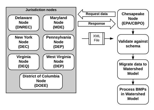
Figure 3 - Illustration of National Environmental Information Exchange Network (NEIEN) process.
