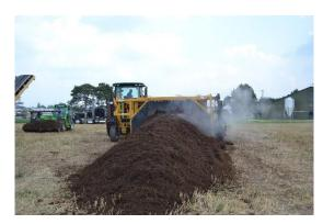
Figure A-14-4. Turned Piles and Windrows rely on frequent turning, usually with specialized machinery, to aerate the compost. Photo: Robb Meinen, Penn State.
