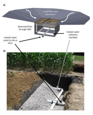
Figure A-21-1. a) Diagram of typical blind inlet and b) cutaway of a blind inlet in the field. Source: Upper image from Penn and Bowen, 2017, lower image from USDA-ARS. See Expert Panel Report (p.18).
