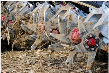
Figure A-17-1. Specialized equipment is used for manure incorporation and injection. Manure incorporation requires machinery that mixes dry, semi-dry or liquid organic nutrient sources – such as manure, bio-solids, and compost – into the soil
