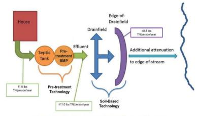
Schematic of a residential septic system with pre-treatment and soil-based BMPs
