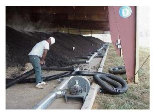
Figure A-14-2. Forced aeration systems, or aerated static piles, use blowers to provide oxygen into the compost pile instead of turning or moving the pile. Photo: Jason Governo, U. of Georgia.
