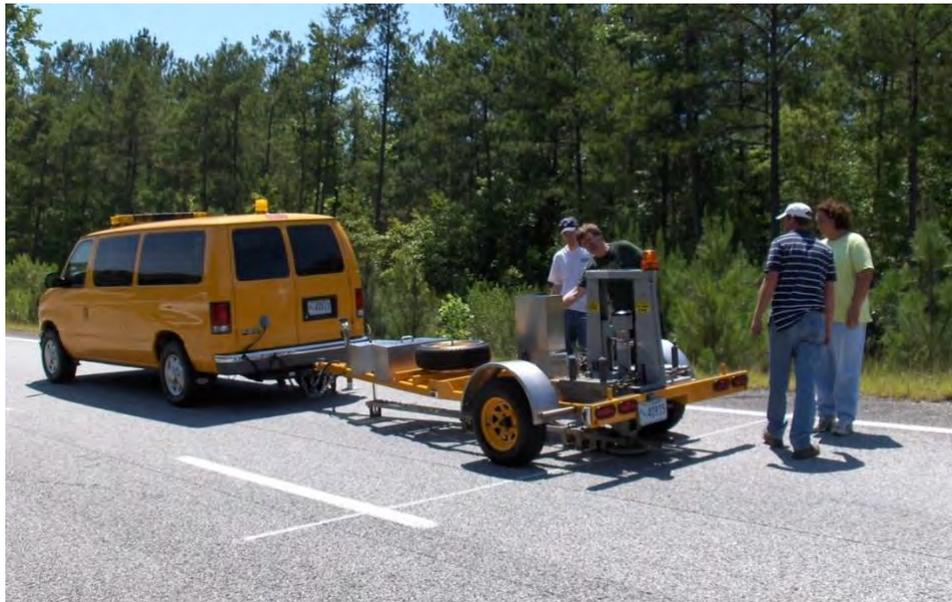
**Figure 7 Dynatest Model 8000 Falling Weight Deflectometer on the Test Track**
