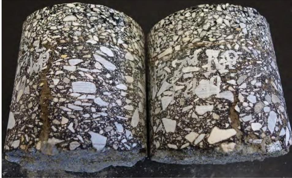
**Figure 15 Section N5 (Standard RAP) Cores Showing Bottom-up Cracking**
