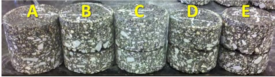
Figure 22 (a) Cores Taken from Section S5 (High RAP) in April 2013
