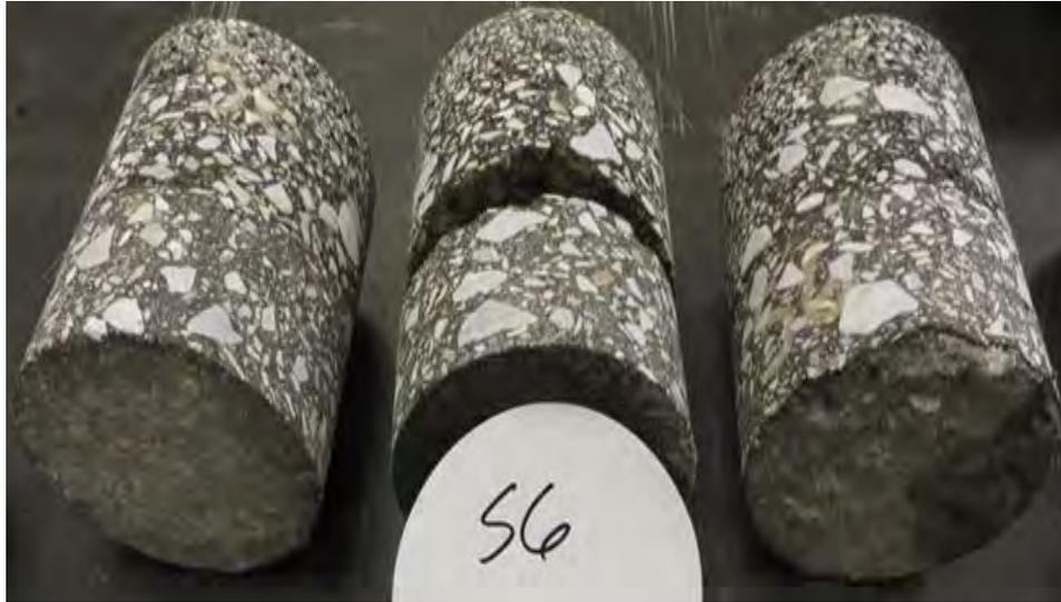
**Figure 31 Cores Taken from Section S6 (RAP/RAS) in September 2013 (1)**
