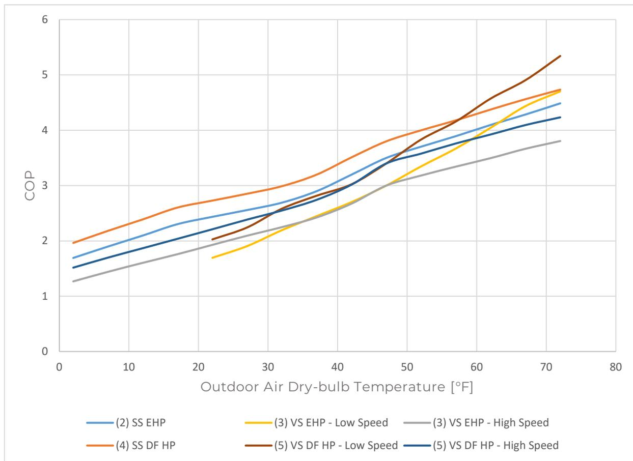
Figure 14 – Heat pump COP at rated indoor air conditions
