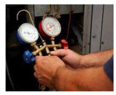
Refrigerant Gauges Not Connected
