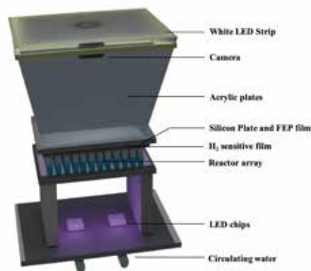
Schematic illustration of the parallelized and automated photochemical reactor (PAPCR) for the high-throughput measurement of hydrogen production. The apparatus sits on bench top.
