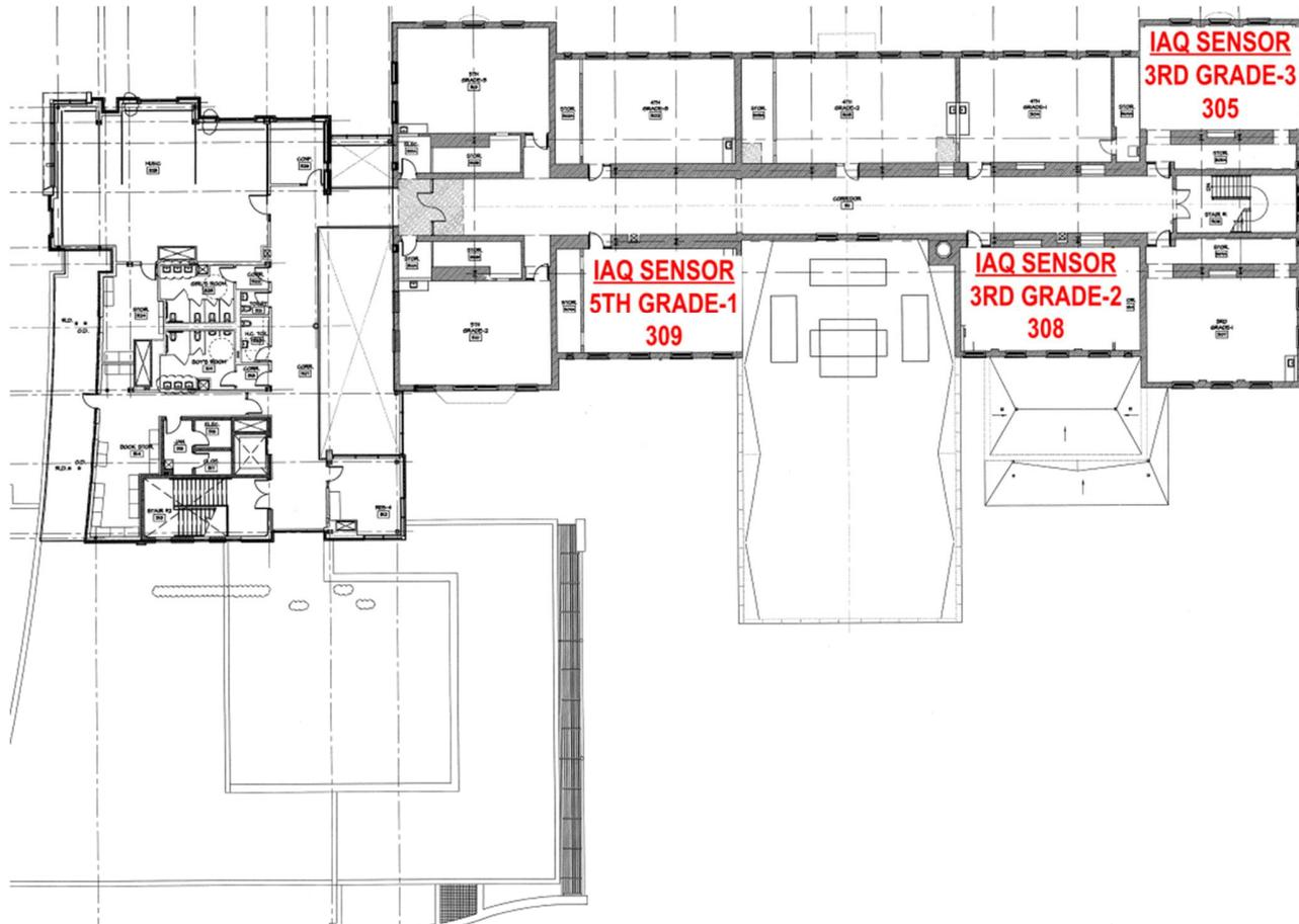
Figure 4.4: IAQ sensor plan – Third floor plan
