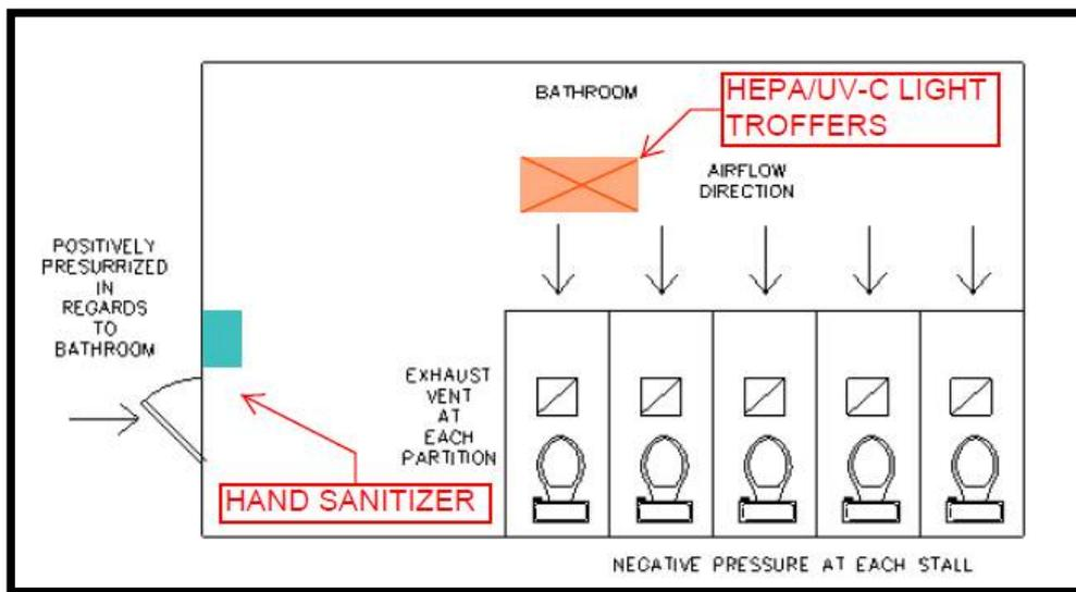
Figure 7.1: Typical Bathroom Layout
