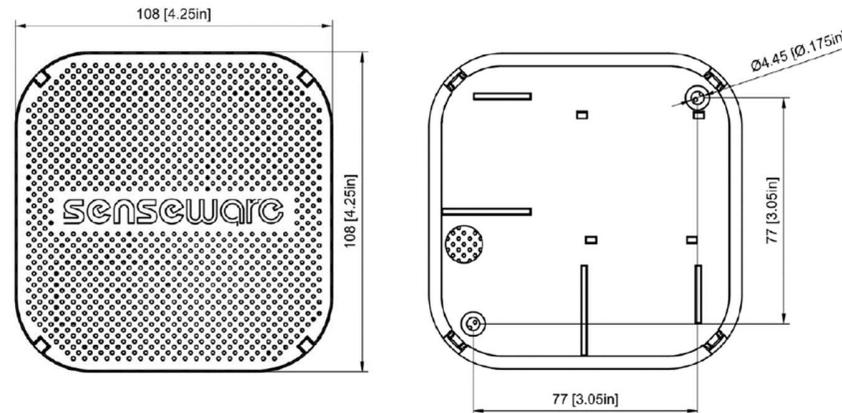
Figure 4.5: Senseware Sensor Picture (Dimensions in mm)
